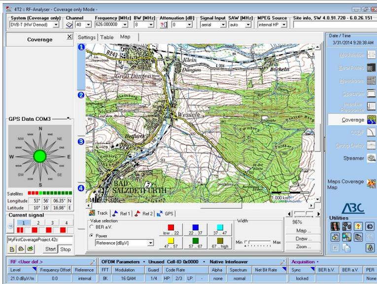
Once the map is loaded, measurement values can be plotted on the map when the measurement is started.
