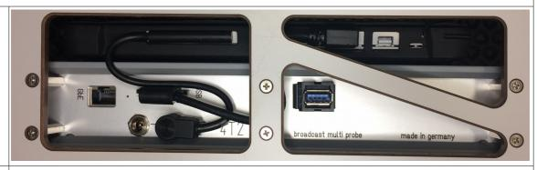
GbE gigabit ethernet connector for networking and transport stream input and/or output streaming
